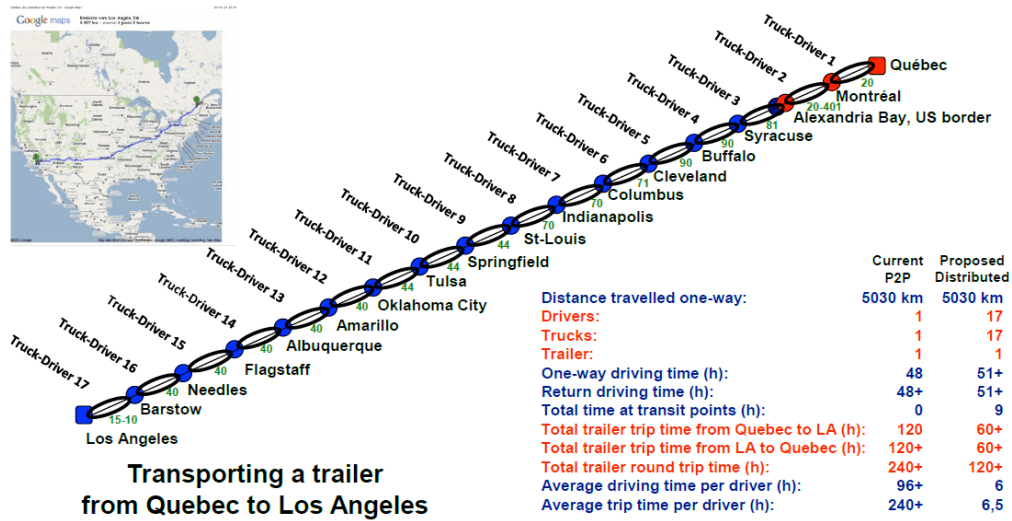
Figure 4.1: Simulation of a trailer transport journey Québec City (Canada) to Los Angeles (USA).
