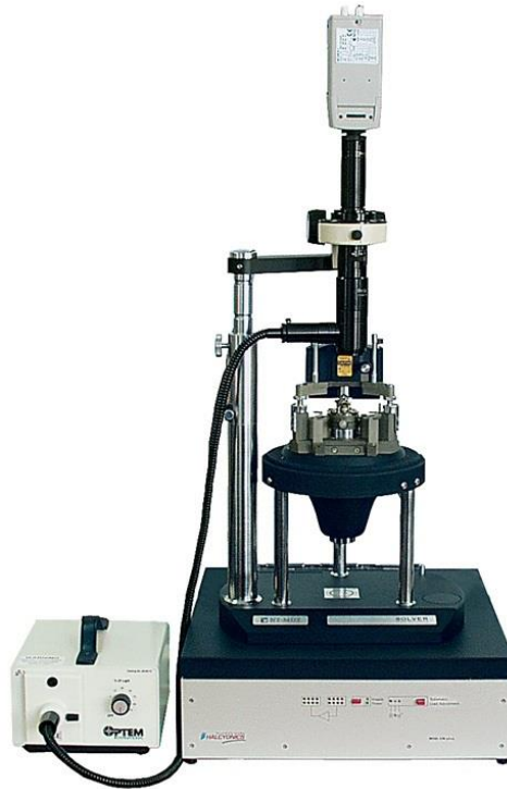
Fig. 3.2.9: image of the AFM Solver Pro-M used to acquire the AFM data. 114
