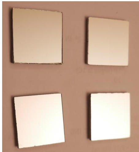
Fig. 6.2.1: image representing some of the square-based (1.5 cm side) samples prepared for the optical and structural characterization.
