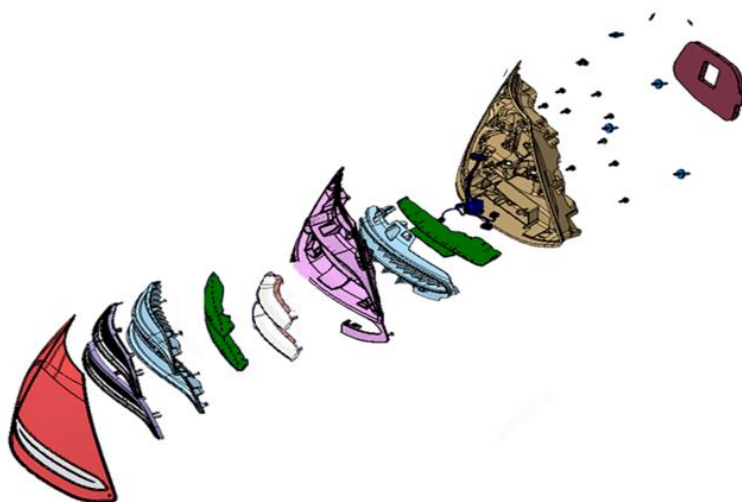
Fig. 1.2.2: exploded view of a rear lamp, showing all its internal components.
