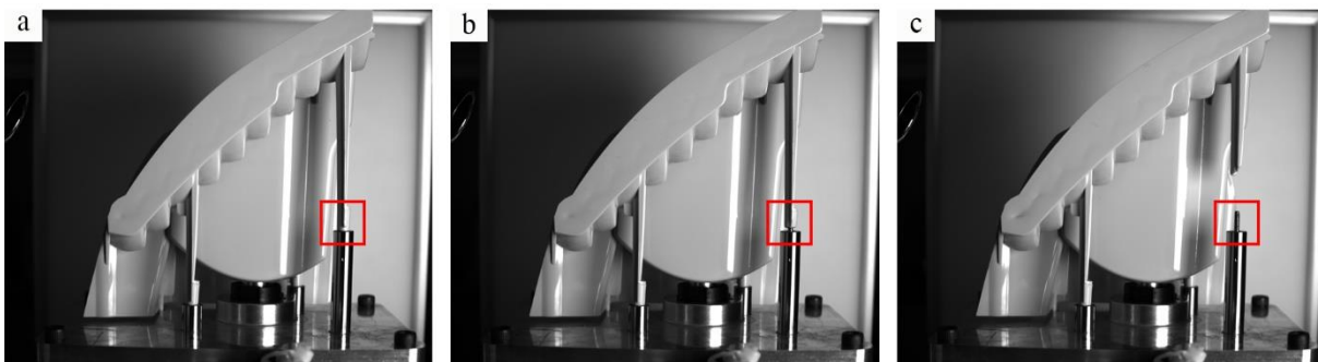
Fig. 6.3.22: example of detection of pin incompleteness. The red rectangle represents an enlargement of the ROI exploited for the pixel intensity analysis, which otherwise would have been impossible to be visualized. It is therefore possible to distinguish compliant (a) and faulty pieces (b, c).
