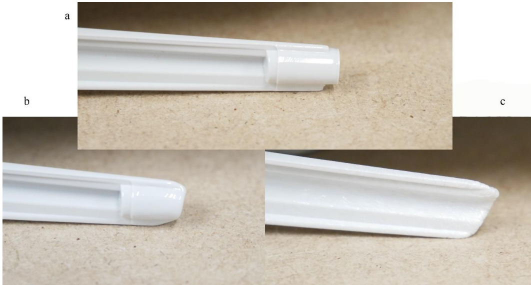
Fig. 6.3.21: example of pin incompleteness. A compliant piece (a) is compared to a pin showing a faint incompleteness (b) and one presenting a severe defect (c).
