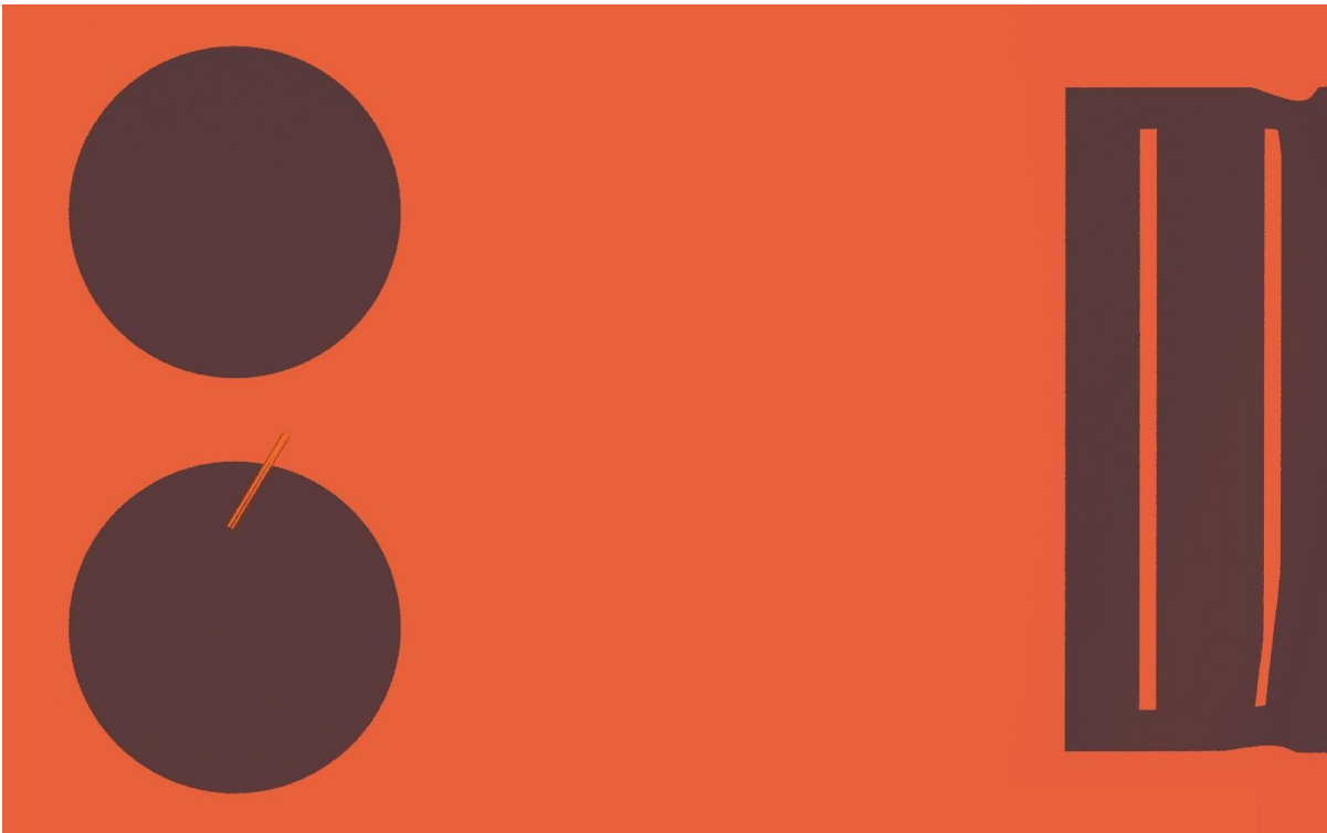
Fig. 5.3.10: back-tracing simulation (8.000.000 rays) of a scratch on the outer lens. The scratch is placed between the dark circle and the white background to evidence the importance of the dark structure in the scratch detection process.
