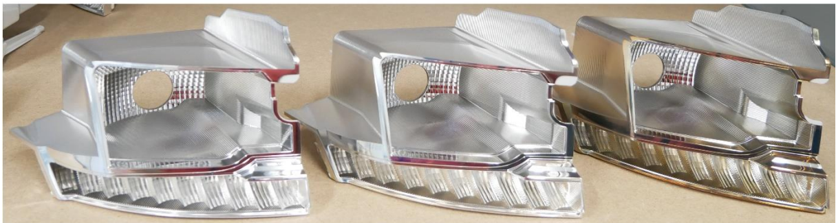
Fig. 6.3.11: example of yellowish. The sample on the left is compliant, while the middle (faint yellowish) and the right (severe yellowish) ones are scraps.
