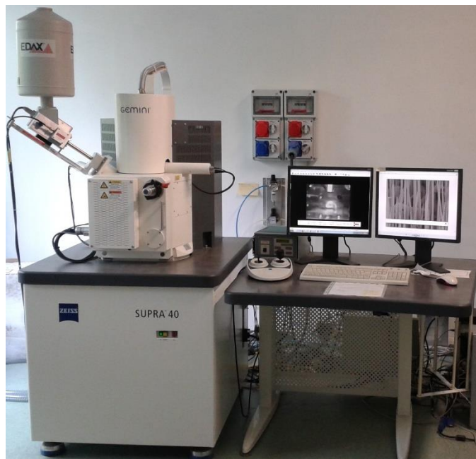
Fig. 3.1.9: experimental setup of the CNR-IOM ZEISS SUPRA 40 SEM used in this thesis.
