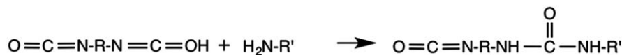
FIGURE 8. Tissue adhesion mechanism of urethane-based adhesive: H 2 N-R' represent tissue amines that react with isocyanate groups through urea bond formation.
