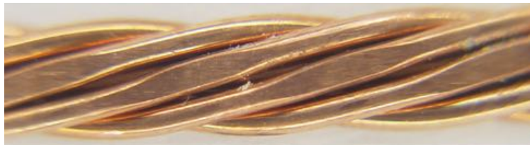
Figure 10.28: Picture of good quality 6 around 1 cable with thickness of 1.72 mm.
