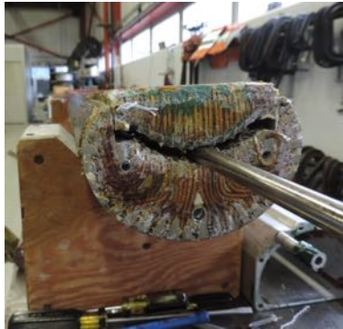
(a) Separating the Coils
