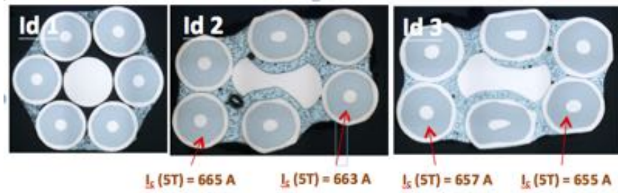
Figure 10.30: Cross sections of NbTi cables made with six superconducting wires around a central Cu strand and showing I_c data at 5 T. (Pictures by Marianne Bossert.)
