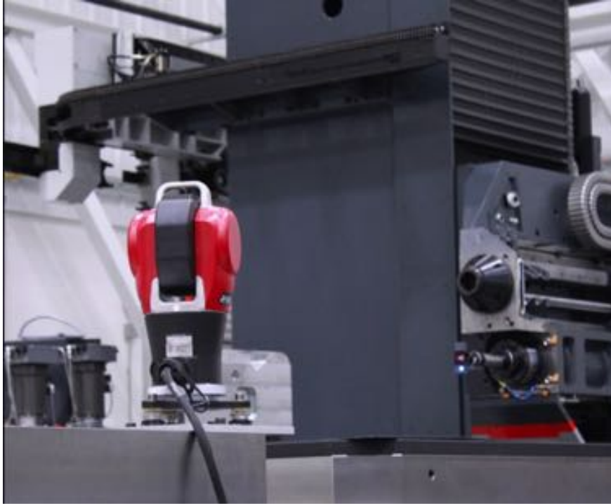
Figure 9.20: The Radian API Laser Tracker System.
