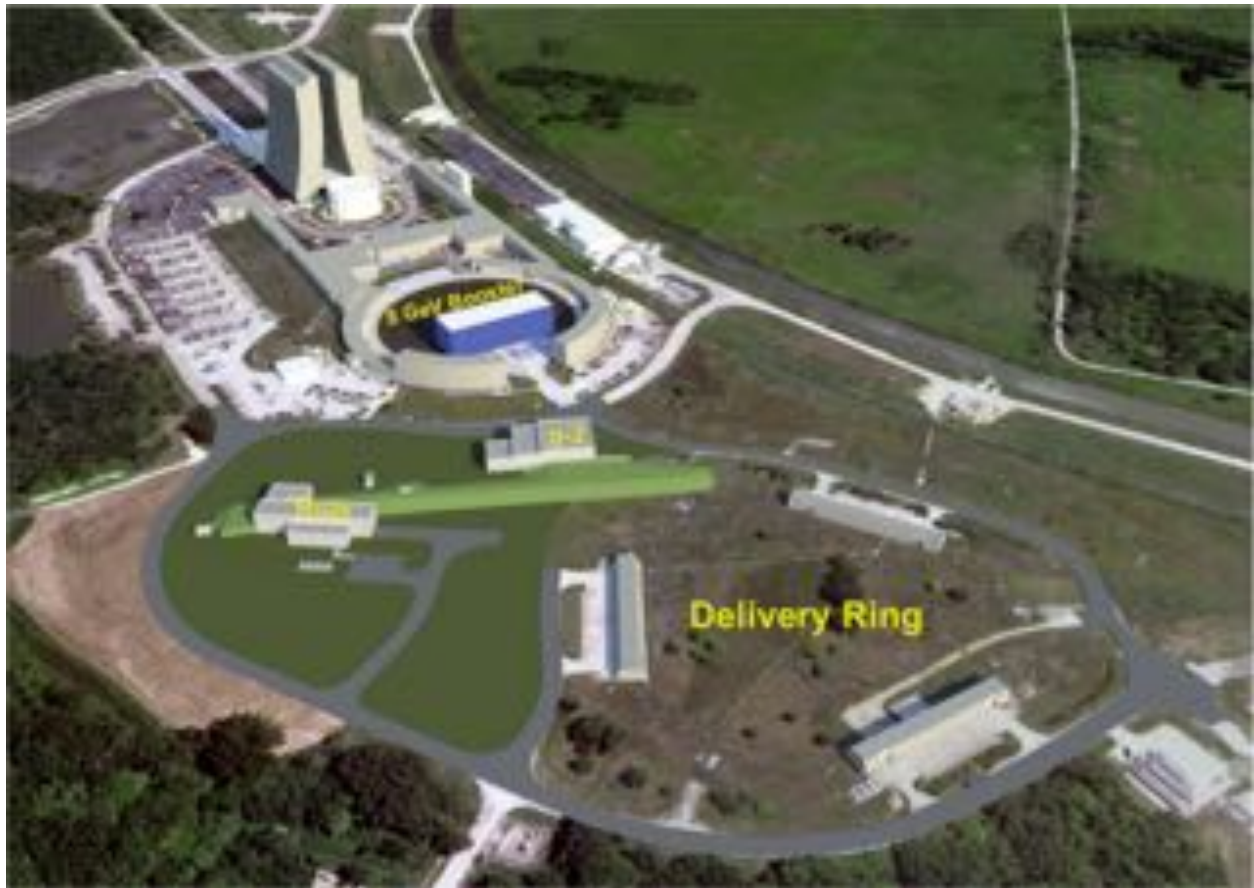
Figure 6.1: The layout of the Muon Campus, which lies between the former Antiproton Rings and the Booster Accelerator. The locations of the (g - 2) and Mu2e experiments are labeled.
