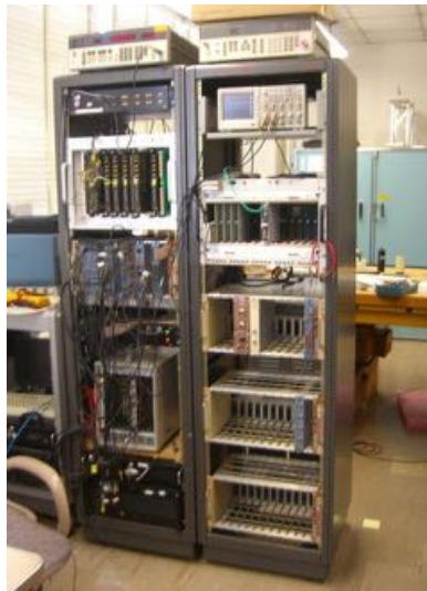
Figure 21.4: Photograph of the DAQ test stand including \mu TCA-based electronics and VME-based electronics at the University of Kentucky.
