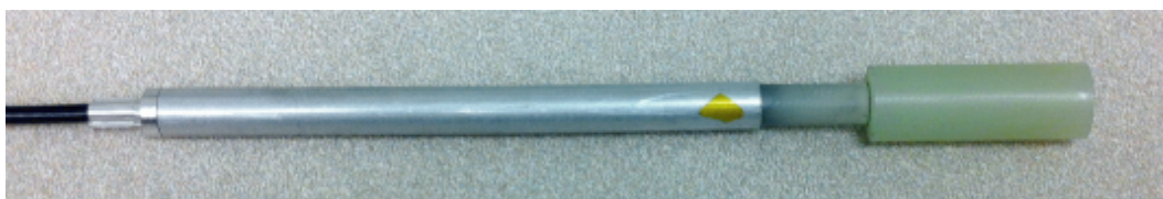
(b) pNMR probe with crimp connection
