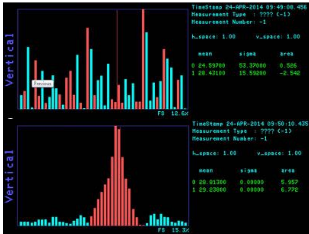
Figure 7.82: Wire profile at the 728 location for 10^{11} 120-GeV protons on target with 2.5 \times 10^8 low-intensity secondary beam measured using an ion chamber at at 728. The top plot is the noise sample and the bottom plot shows the results of subtracting the noise sample from the raw beam signal.
