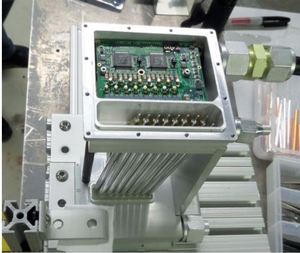
Figure 19.21: ASDQ boards mounted inside the manifold of the 32 channel prototype
