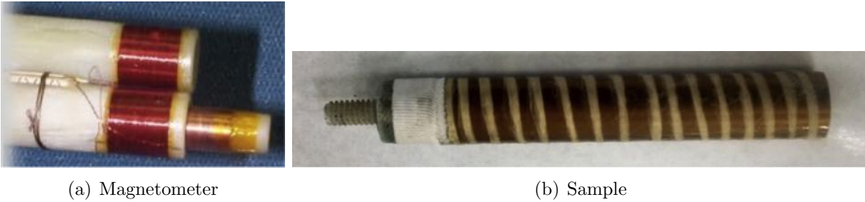
Figure 10.38: (a) Balanced coil magnetometer used in TD to measure magnetization of superconducting samples. (b) Magnetization sample made by winding a number of turns of the NbTi Luvata foil.
