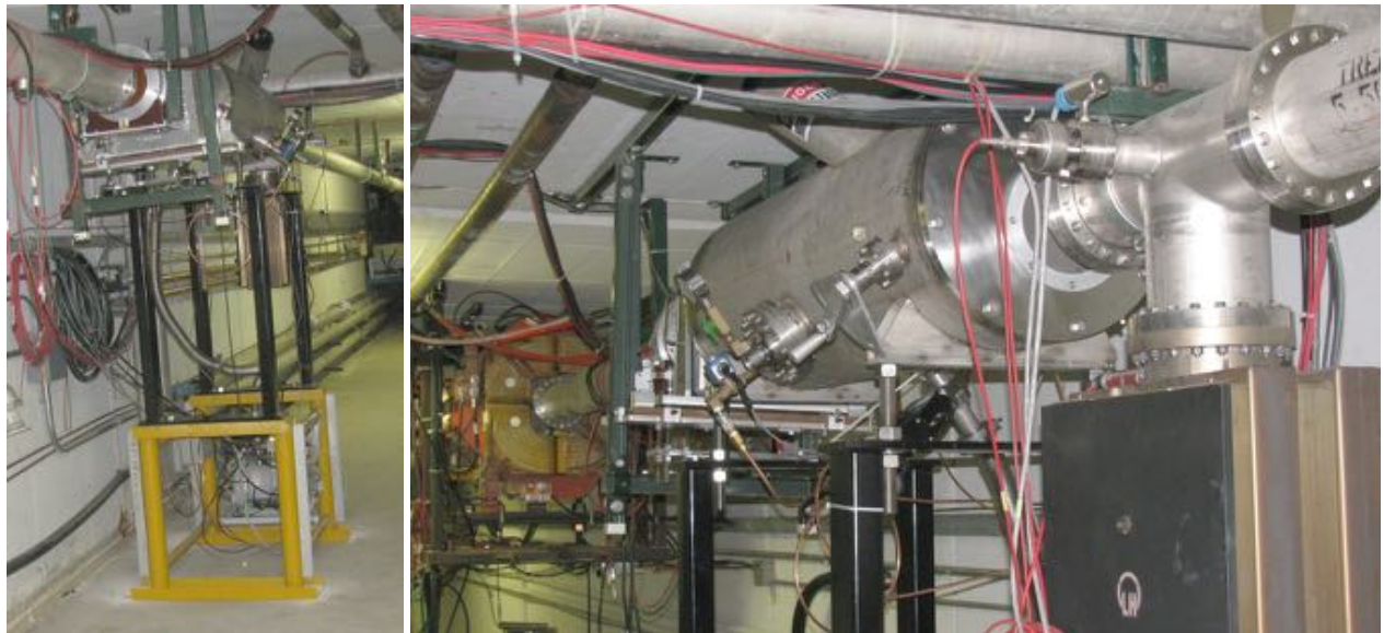
Figure 7.87: Cerenkov detector installed in the AP2 line.
