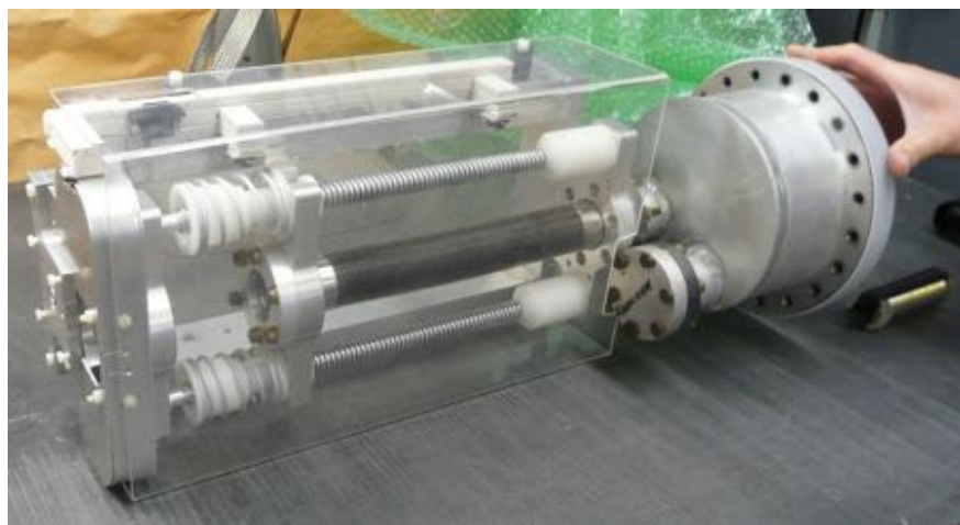
Figure 11.6: The plunge probe mechanism. The probe lies inside the titanium vacuum bellow.
