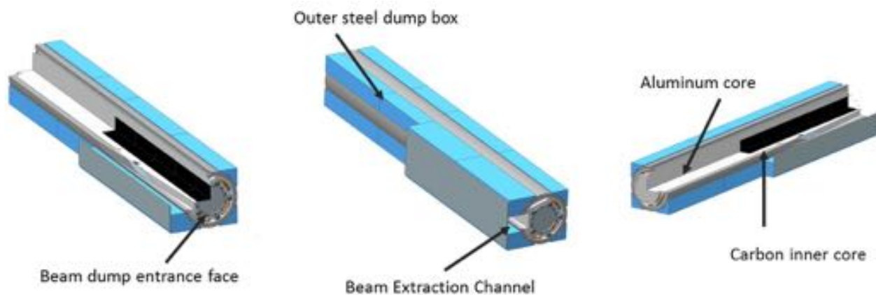
Figure 7.23: Design of the AP0 beam dump core.
