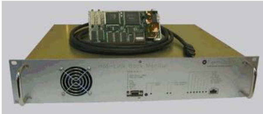
Figure 7.70: A Hot-Link Rack Monitor is a flexible data acquisition system composed of a remote unit and a PCI Mezzanine card that resides in a VME crate. Each HRM provides sixty-four 16-bit analog input channels, 8 analog output channels, 8 TCLK timer channels and 8 bytes of digital I/O. HRMs will eventually replace all of the functionality of CAMAC [30].
