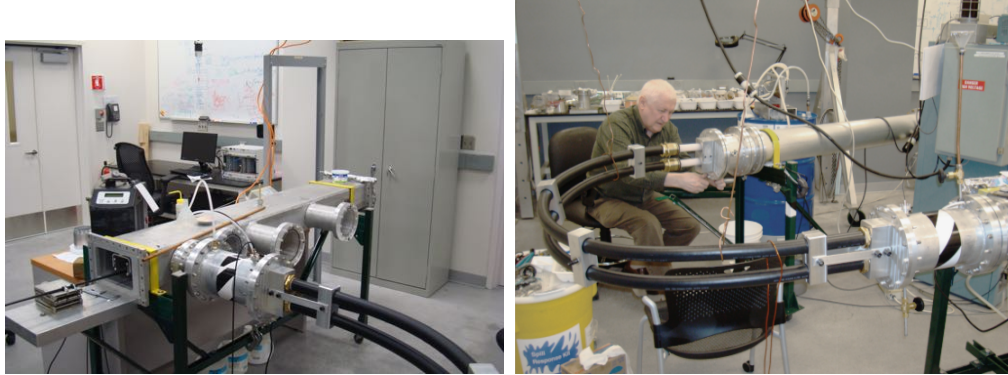
Figure 12.16: (Left) Vacuum chamber with prototype kicker plates installed. The plates are just visible inside the end of the chamber. A magnetic field probe, mounted on a movable stage, is inserted between the plates. (Right) Downstream end of the Blumlein and pair of 50\Omega coaxial high voltage cables, (Times Microwave Systems AA-8740 - RG220/U equivalent) couple Blumlein to kicker plates.
