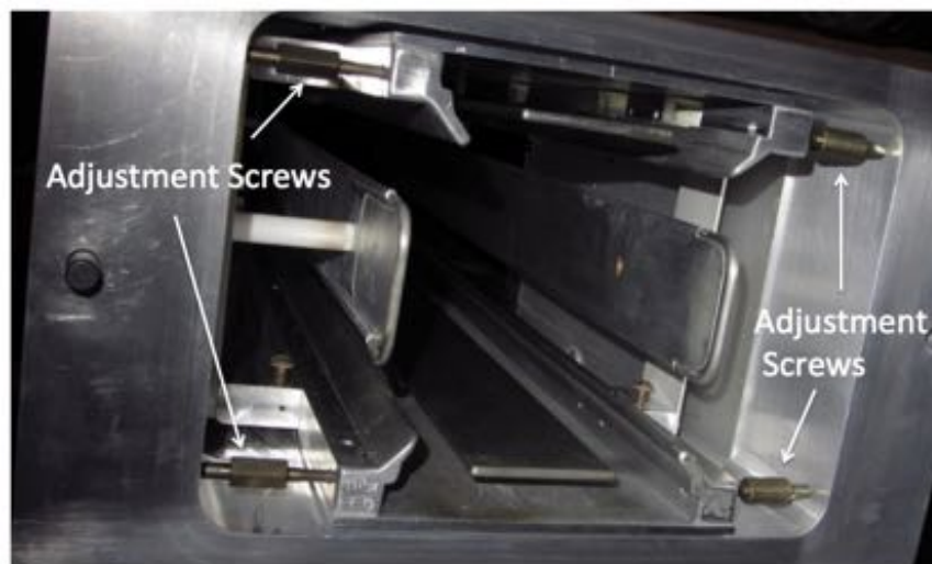
Figure 11.3: Picture of a cage system showing the (1) quadrupole plates, (3) macor (insulator) supports, (4) trolley rails, and (5) a wheel for guiding the cable that pulls the trolley
