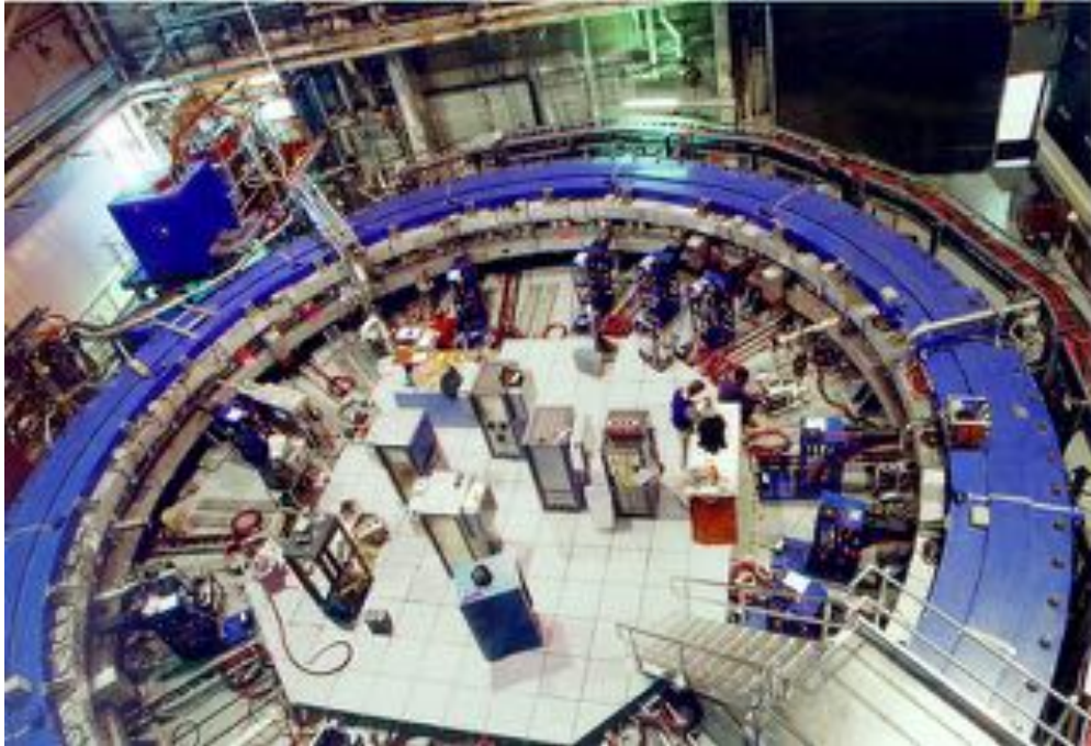
Figure 3.1: The E821 storage-ring magnet at Brookhaven Lab.
