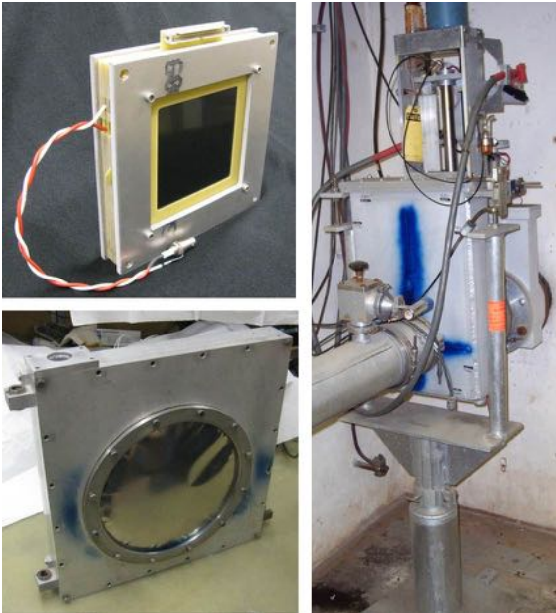
Figure 7.86: The first completed PWC prototype (top left). The signal connection is at the top and the high voltage connection comes out the left side. The PWC is installed in an anti-vacuum box (lower left). ArCO 2 gas is pumped into this chamber, and there is a vacuum window on both front and back of this module. The anti-vacuum chamber is installed inside of the bayonet can (right) which is pumped down to beam tube vacuum. The PWC wires can be lowered into the beam or raised out of the beam via a motor drive.
