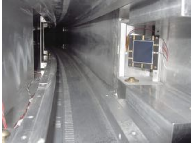
Figure 10.13: A photo of the inflector cryostat exit. A silicon detector (in blue) measured the beam profile just downstream of the inflector cryostat exit
