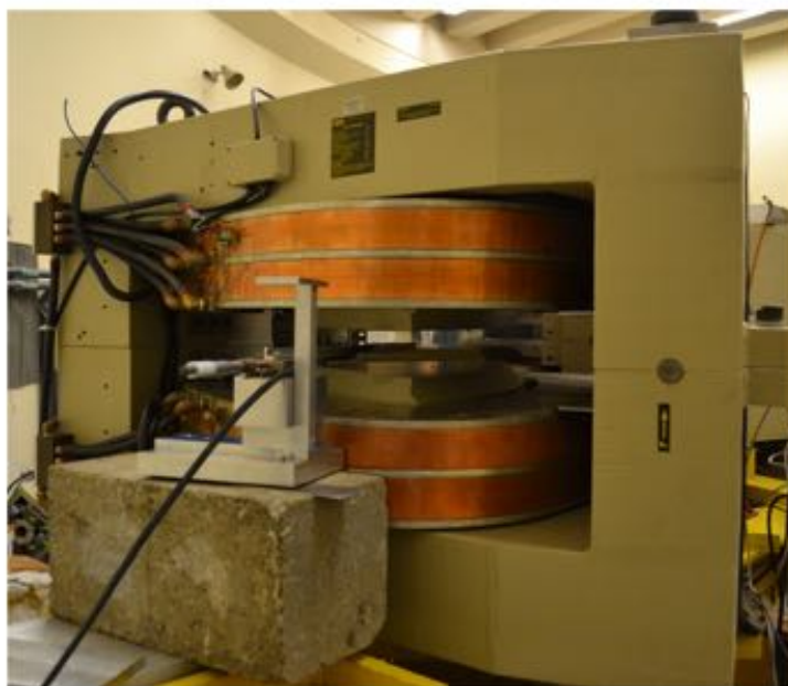
Figure 15.4: Dipole magnet at the University of Washington shown with field mapping in progress. It provides a 1.45 Tesla field sufficiently uniform for testing probes and electronics for the E989 fixed probe system.
