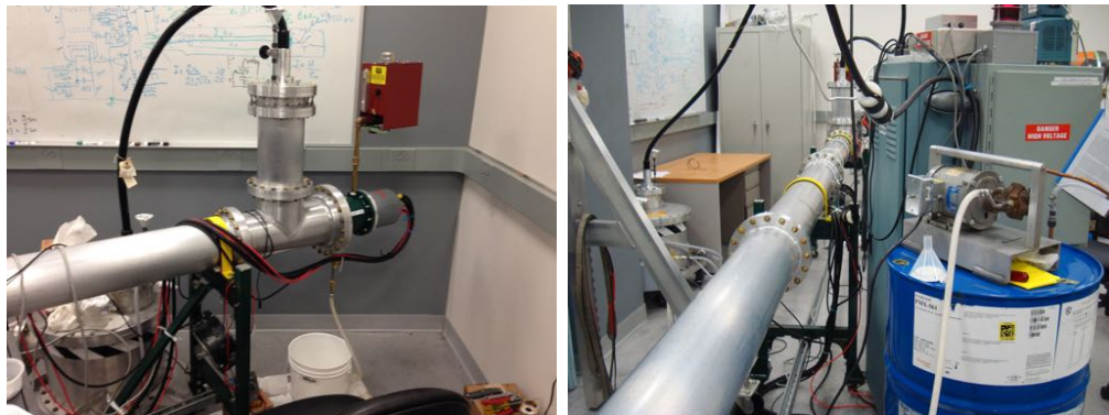
Figure 12.15: (Left) Upstream end of Blumlein. The black cable attached at the top of the transition delivers the charging current. The CX1725X thyatron is mounted horizontally in the far right (green) module. The space between the conductors of the Blumlein and the volume around the thyatron is filled with transformer oil. (Right) Looking from the business end of the Blumlein upstream towards the thyatron.
