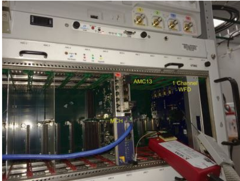
Figure 18.4: The Cornell \mu TCA test stand based on the VadaTech 892, populated with a CMS AMC13 (upper of center pair of modules), a NAT MCH (lower of the central pair), and one of the one-channel WFD prototypes (at right) under testing.
