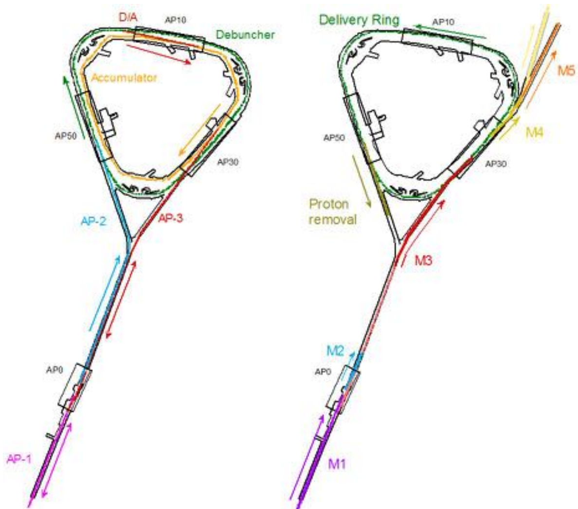
Figure 7.25: Layout of the Antiproton Source beamlines (left) and the reconfigured beamlines for (g - 2) operation (right).
