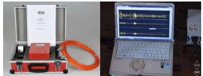
Figure 6. Left: GeoBox SR04S3. Right: the device connected with the computer at work for investigating vibrations in the basement of the castle.
