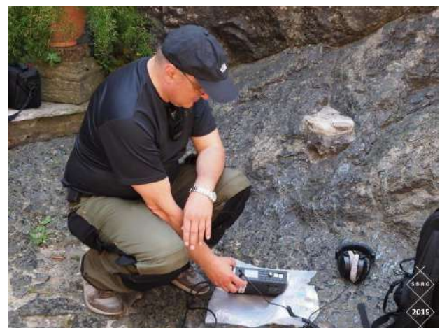
Figure 3. The set-up used for recording sounds: the recorder Tascam DR-680 and microphones Sennheiser MKH 8020.
