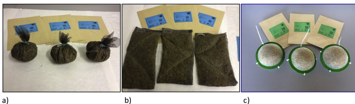
Fig. 2. Different shapes of moss bags tested. a) Rounded; b) Flat; c) Mossphere.
