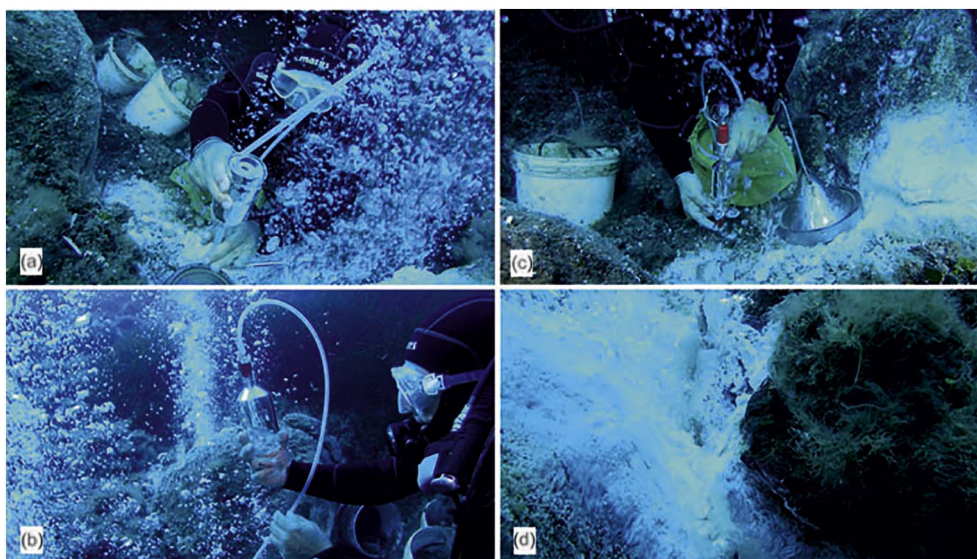
Fig. 2. Pictures illustrating the sampling of warm thermal waters (a,b) and dry gas phase (c) for mercury speciation and major chemical determinations. White bacterial mats deposits (d) often marks the submarine hydrothermal emissions at Panarea Island.
