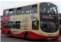
City Line Diesel-Hybrid Bus Engine: 161 kW + 120 kW (el.) Eu V (DOC+DPF+SCR) City Line Profile
