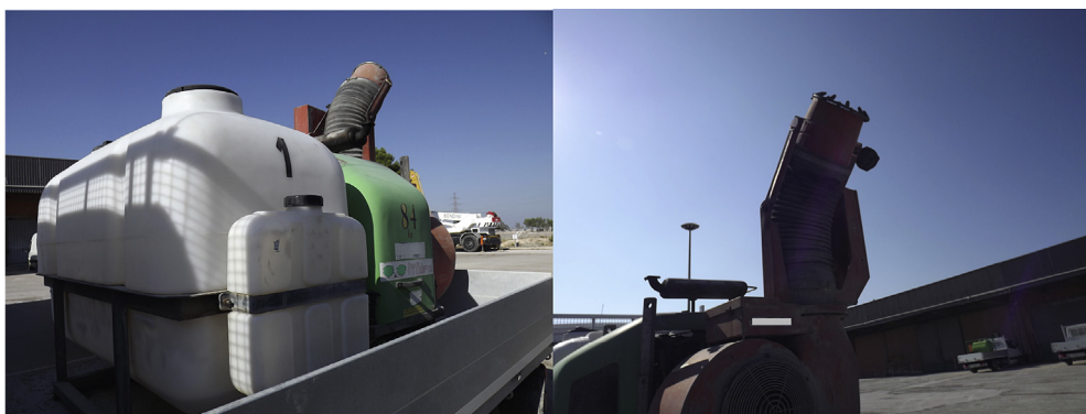
Fig. 3. Atomizer used in the abatement experiment (left), with details of the nozzle (right).
