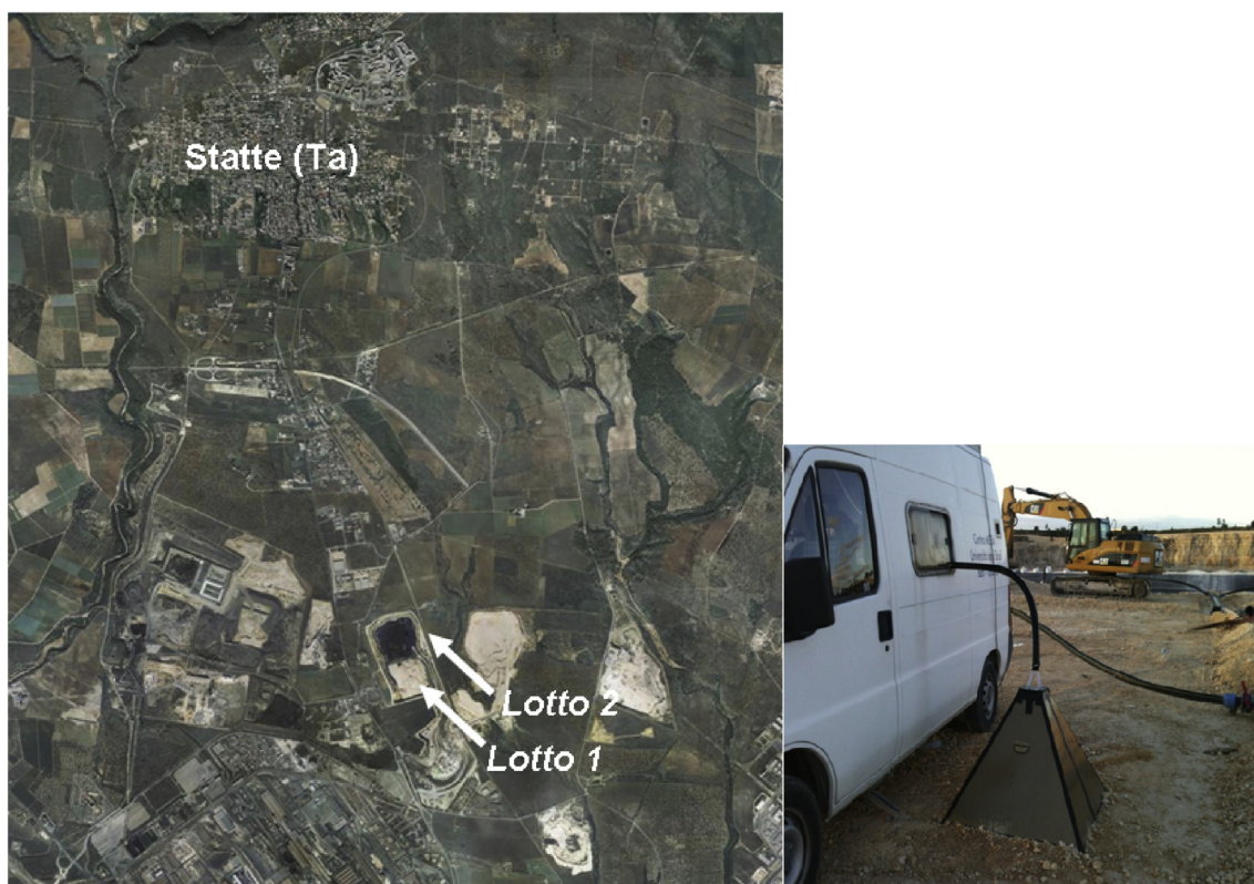
Fig. 1. Left: Italcave waste management plant “Lotto 1” where are located the biogas collection wells and “Lotto 2” the active batch in which are located the wastes under work, the city of Statte (Taranto province) and surroundings (source: SIT Puglia, http://www.sit.puglia.it/ ). Right: static extractor in the “lotto 2” waste management plant field.
