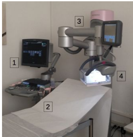
Figure 2.13: picture of the Siemens ABVS equipment: (1) scan station; (2) table for patient scanning; (3) flexible arm; (4) scan head assembly for the 3D imaging.
