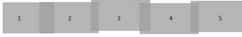
Figure 4.5: Example of a possible small misalignment that will be compensated correlating the information in the overlapped regions.
