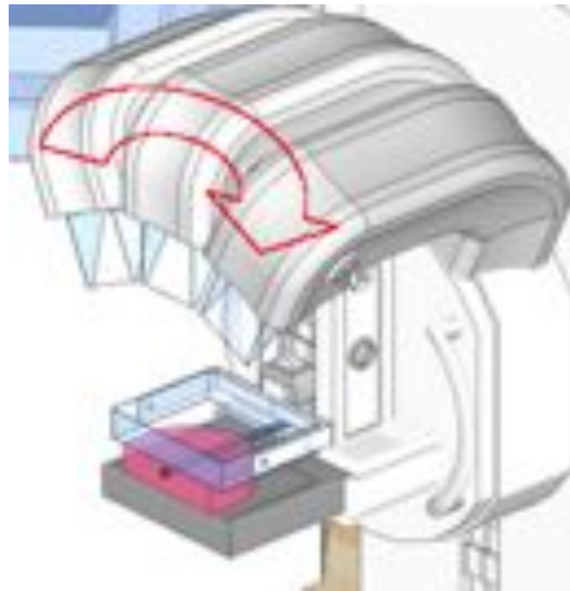
Figure 2.8: sketch of the DBT rotating gantry with respect to the breast position.
