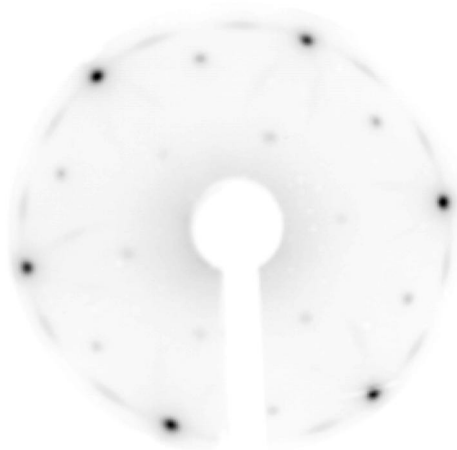
Figure 4.8: LEED diffraction pattern for the Gr/Ni 3 Al(111) system acquired at 71 eV.
