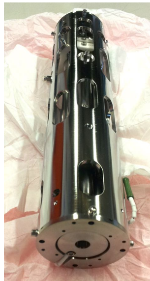
Figure 6.11: Photo of the 16000 a.m.u. Extrel QMS which will be installed in the cluster source.
