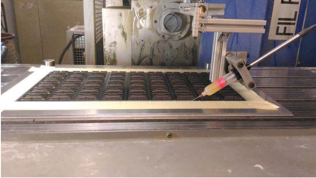
FIGURE 7.25: Putting glue to the MicroMegas PCB with special machine;
