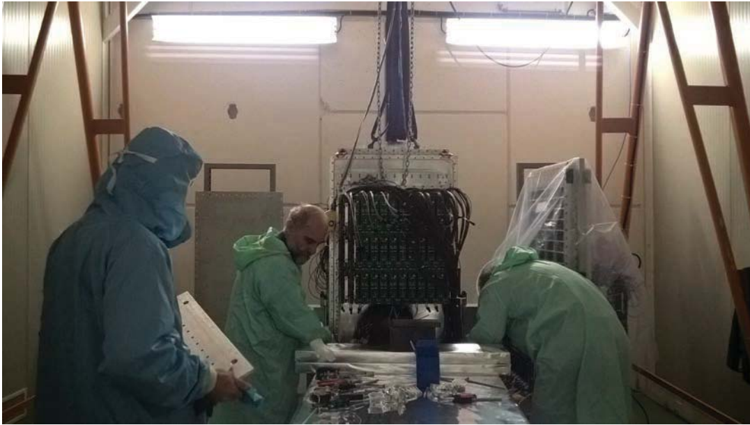
FIGURE 7.54: Preparing the MAPMT part for being dismantled from old frame.
