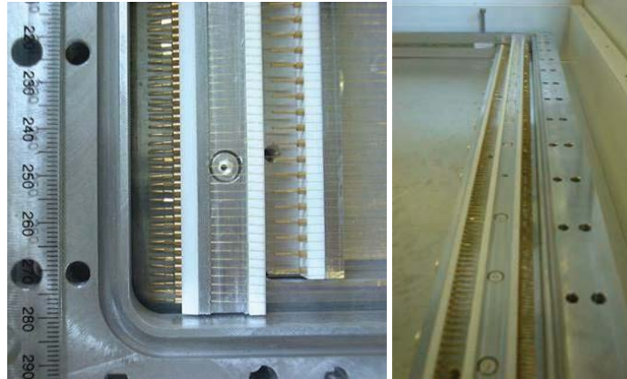
FIGURE 3.15: The structure and some details of RICH-1 MWPCs.
