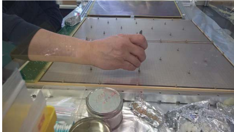
FIGURE 7.46: Putting the spacers before mounting of the THGEM-2
