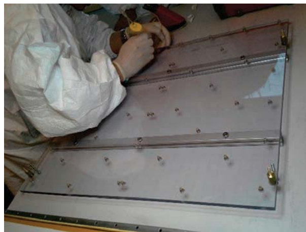
FIGURE 7.30: Mounting of PEEK pillars to the special frame
