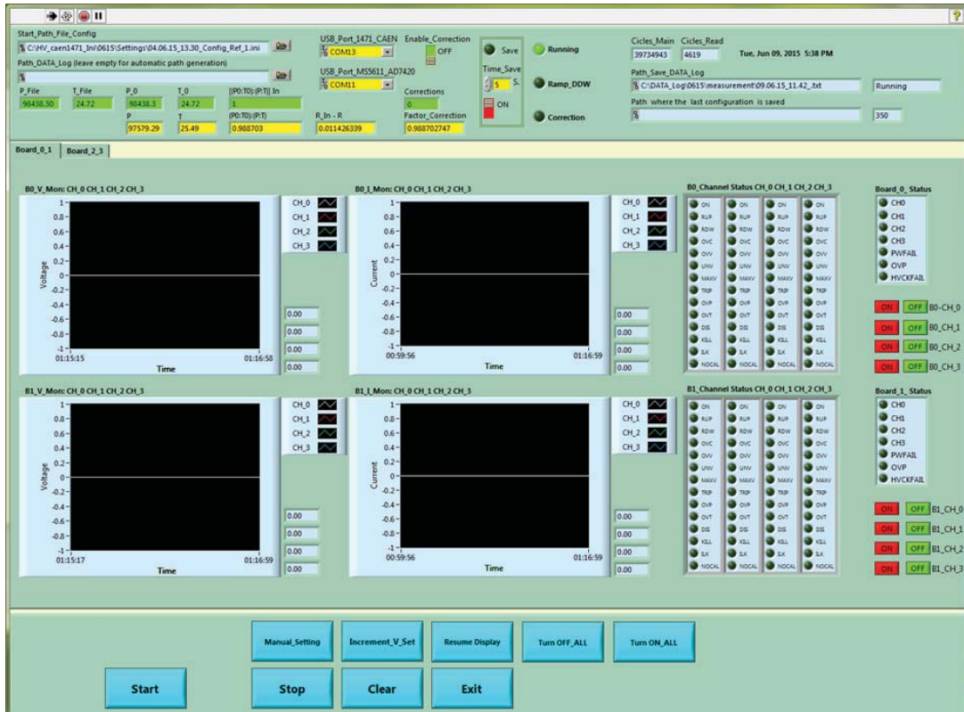
FIGURE 6.33: Custom build LabVIEW based control interface to control effective gain of the chamber with PT variation
