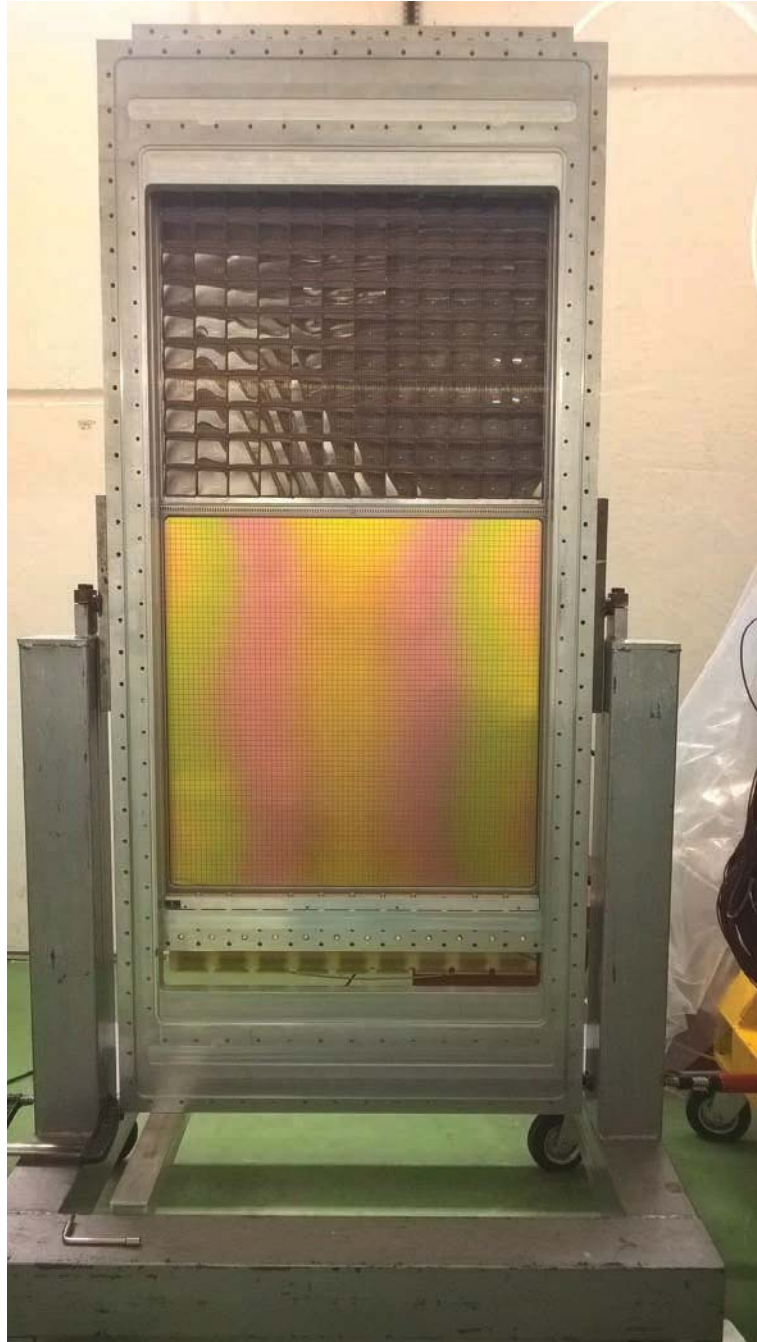
FIGURE 7.53: The old frame with MWPC with CsI photo-cathode (bottom part) and MAPMTs with fused silica lenses (top part), in CERN clean room facility
