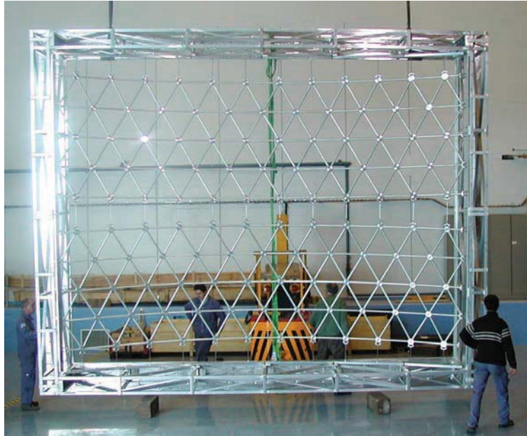
FIGURE 3.10: Picture of the mirror support structure: the nodal points are connected by light Al pipes
