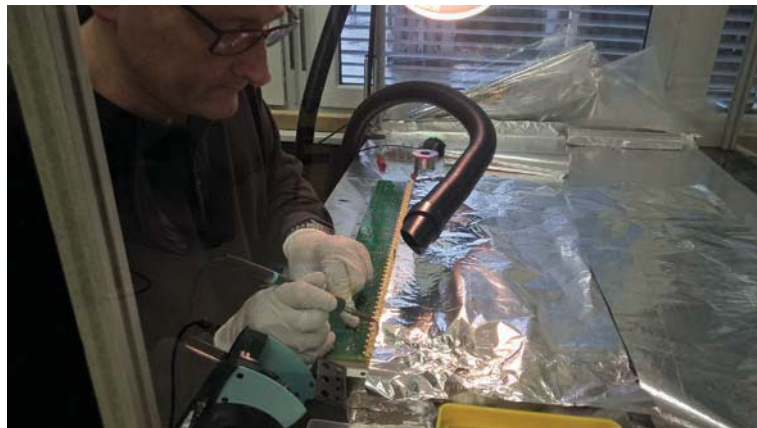
FIGURE 7.47: Mounting of THGEM-2 on the hybrid frame inside a dust free tent
