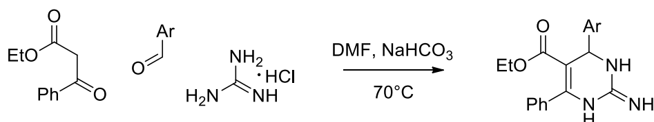
Scheme 15. Synthesis of 4-aryl-3,4-dihydro-2-imino-6-phenylpyrimidines-5-carboxylates proposed by Milcent.
