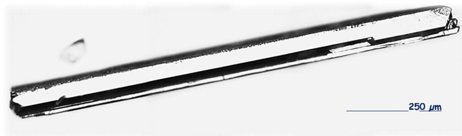
FIGURE 2.9: typical needle-shaped NTI single crystal showing the typical flat surfaces obtained growing the semiconductor in THF
