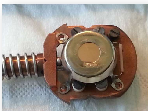
FIGURE 4.21: On the left, the cleaned Au electrode mounted inside the sample holder to be inserted into the UHV chamber. On the right, a typical micrograph obtained for the substrate.
