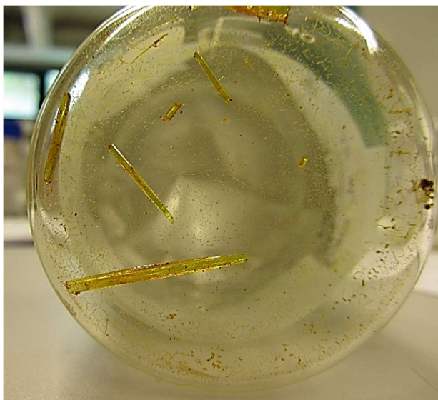
FIGURE 2.13: visible orange inclusions inside MY crystals.
