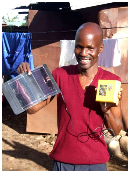
FIGURE 1.2 Accessible electronics: The Pay-as-you-go organic solar cell technology is being distributed throughout rural areas of southern Africa and elsewhere, providing a low-cost and safe alternative to kerosene. Source: Eight19
