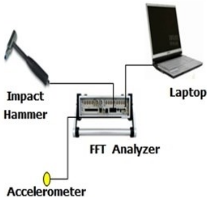
Figure 40 – Setup for the Experimental Modal Analysis
