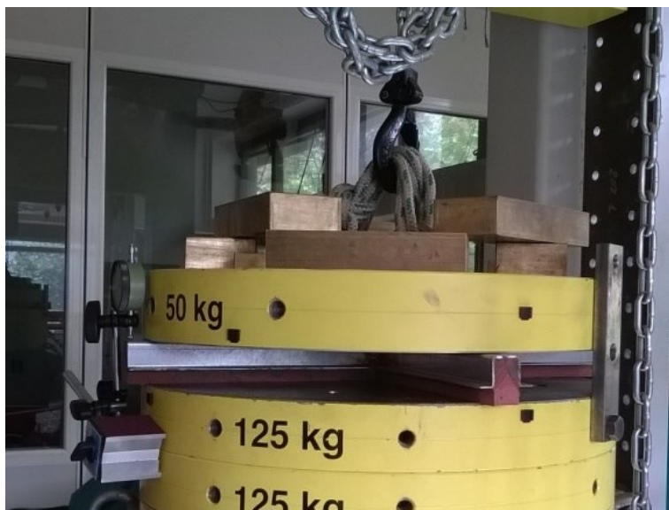
Figure 32 – Setup of the static deflection tests undertaken in laboratory on the floating floor prototypes
