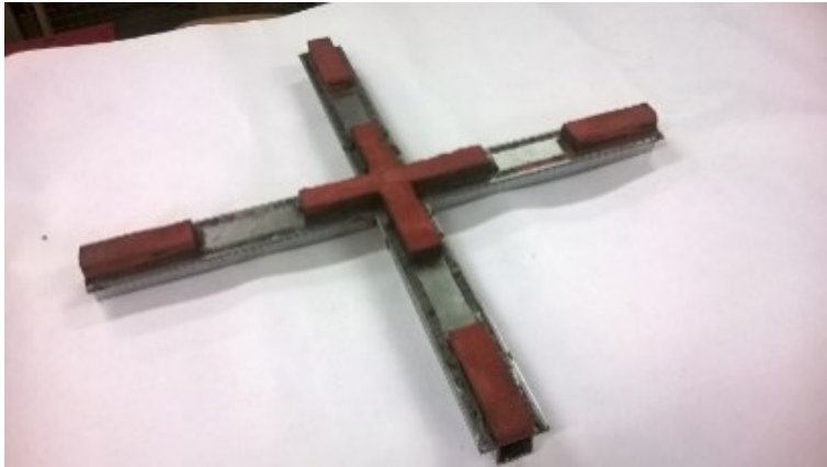
Figure 31 – A floating floor prototypes built after the numerical simulations
