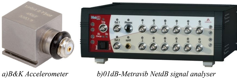
Figure 65 – Acquisition system elements
