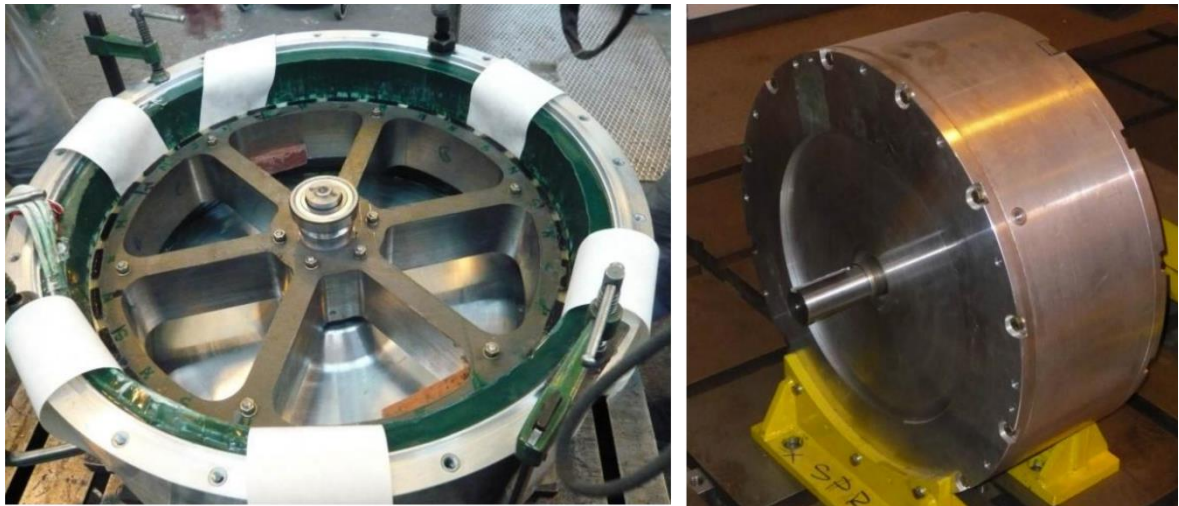
Figure 25: Slotless SPM machine example with and without enclosing shields
