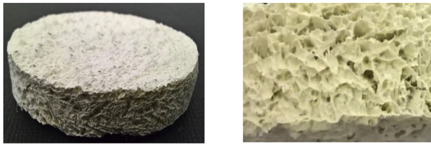
Fig. 1. Example of not-sintered glass foam and a macro structure detail (sample 10).
