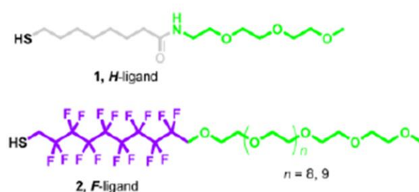
Figure 16: chemical structure of the PEGylated F- and H- ligand
