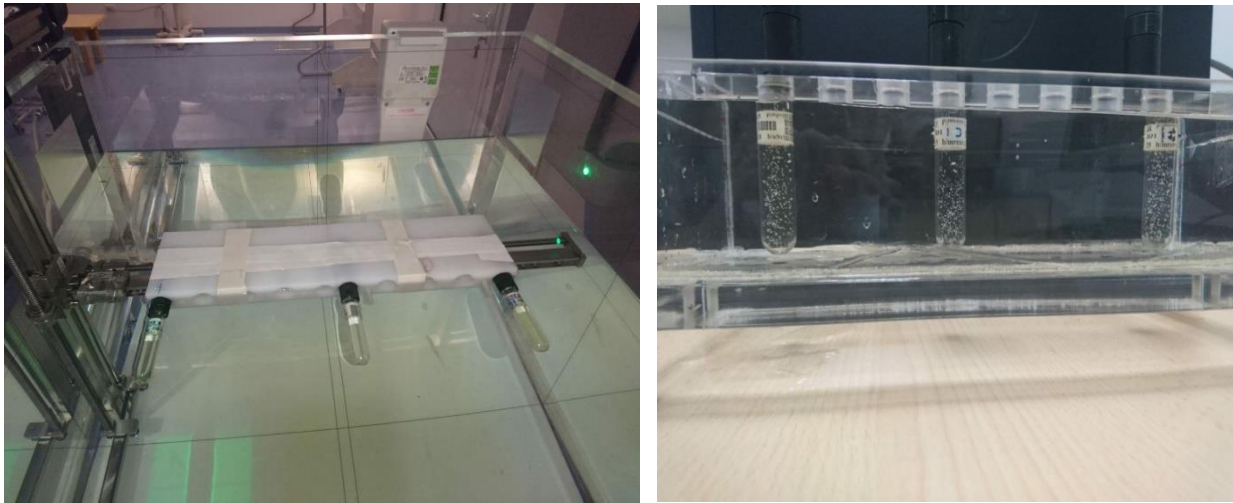
Figure 23: The bubble detectors placed and fixed in arm of water tank using a special holder. The bubble detectors placed inside the beam, 15 cm and 30 cm out of the field at two depth of 1cm in which pacemaker is usually implanted. The SSD was 100cm, field size was 10x10cm of 15 MV photons.
