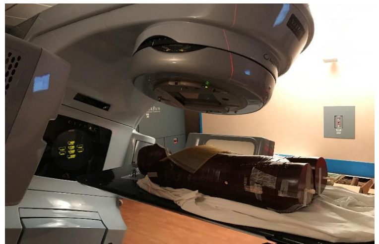
Figure 7: Experimental setup with a 1-cm thick bolus-(C1:top right, C3: bottom right).
