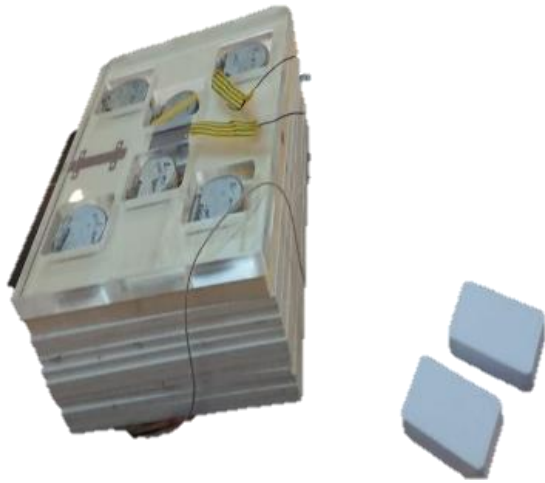
Figure 13: (Left) The experimental setup; (Right) top view of the acrylic slab designed to position the ICDs into six specific holes. Four holes were designed to be 3 cm away from the planning target volume (PTV), and two holes were designed to be placed partially inside the PTV.
