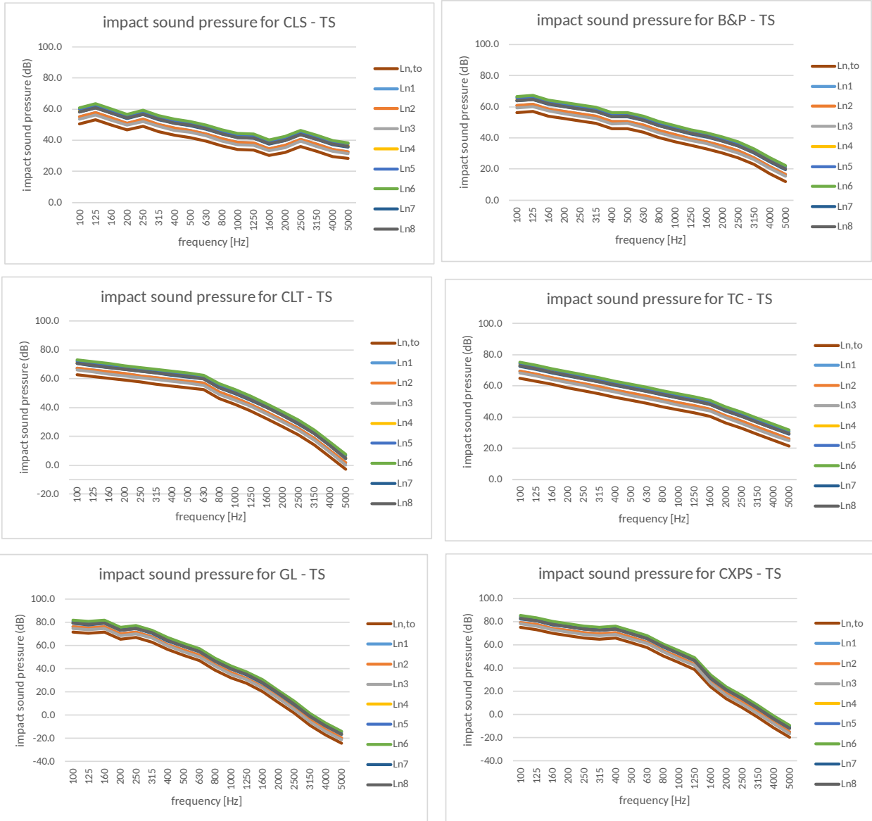
Figure I - normalized impact noise for 6 bare floors with floating floor using TS at different time steps
