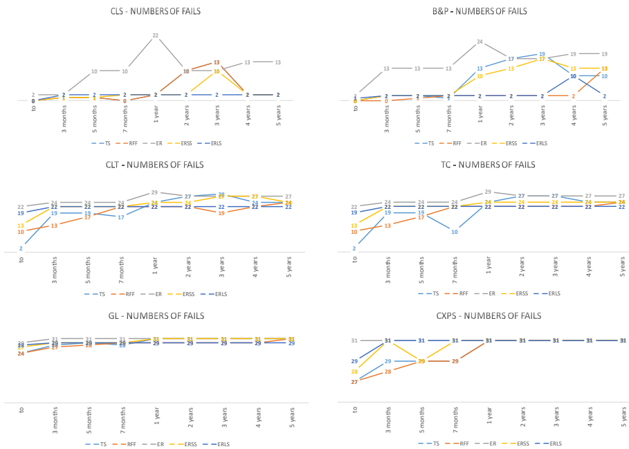
Figure 11 – Percentage of fails for different bare floors with floating floor referred to European regulations.
