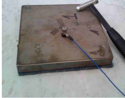
Figure 4 - Apparent dynamic stiffness test measurement facilities.
