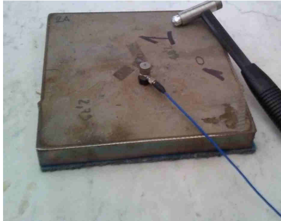
Figure 4 - Apparent dynamic stiffness test measurement facilities.
