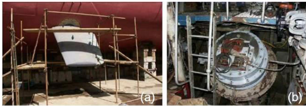
FIGURE 7. (a) Stabilizing fins for a naval vessel and (b) detail of the skull-mounted hydraulic steering system.
