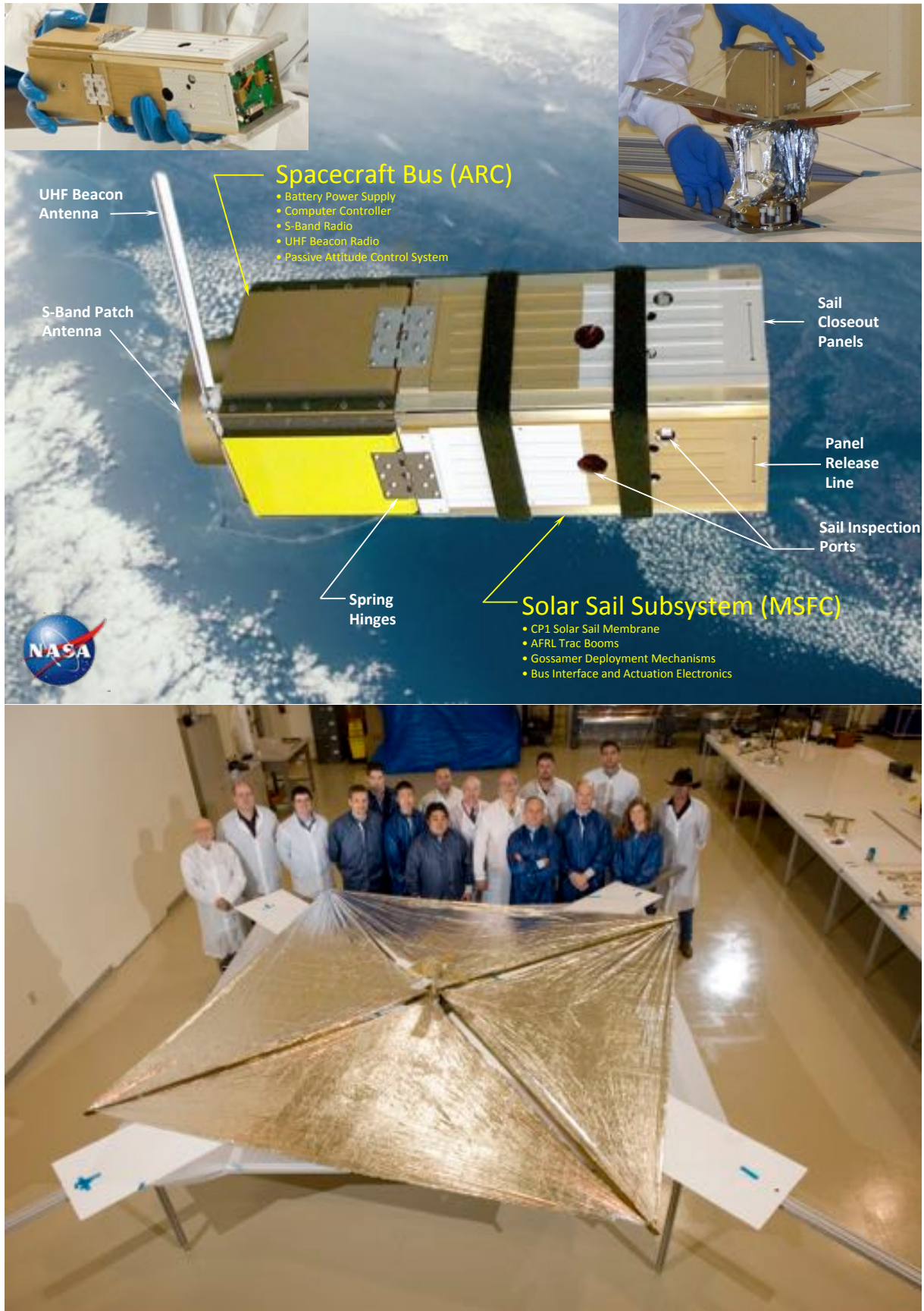
Figure Error! No text of specified style in document..24: Top: on-orbit view of the NanoSail-D2 spacecraft before sail deployment (image credit: NASA/ARC). Bottom: Panel deployed configuration of NanoSail-D (image credit: NASA)
