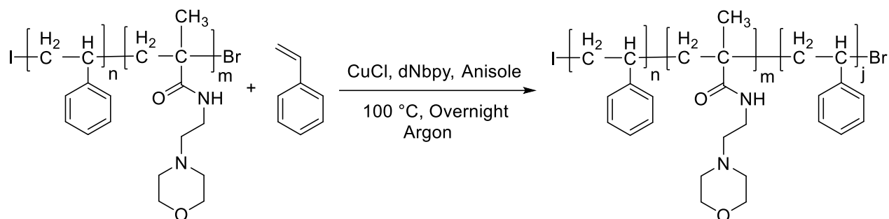
Scheme 9.6 - Synthesis of polystyrene- b -[poly-2- N -morpholinoethyl methacrylate]- b -polystyrene triblockcopolymer
