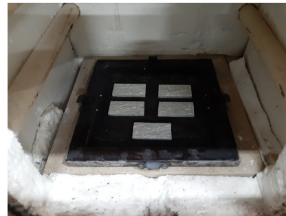
(b) After calcination at 600 °C
