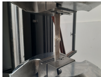
(b) Broken Ax.2 sample
