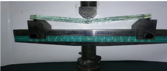
Fig. 8. Three-point bending performance assessment of LG specimens.
