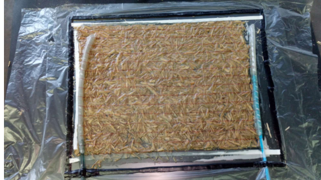
Fig. 5. Vacuum sealing process and the resin adduction device.
