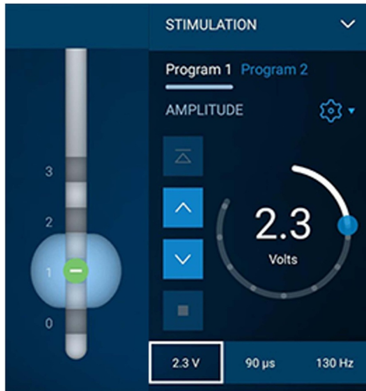
Figure 4. Visual representation of the volume of tissue activated (VTA). The programming user interface of Medtronic ( left ) and Boston Scientific ( right ), showing the VTA as a virtual reproduction in 3D of the spread of current (electrical field) delivered by the DBS lead to the anatomical structures near the selected target.
