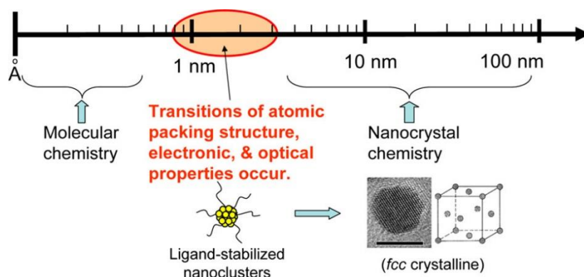
Figure 1.32. Metal clusters placed in a dimensional scale between NPs and molecules. Reproduced with permission from ref. 8. Copyright 2009 Royal Society of Chemistry.
