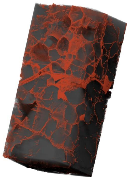
Figure 5: 3D reconstruction of a volume of interest in sample MG10x obtained at step C (see text and Table 1), 1585x1453x3322 voxels. The red phase is serpentine, which fills fractures and intergranular spaces.
