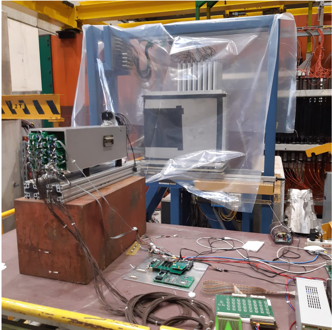
Figure 7.2: HVPSS used as voltage control to polarize 25 PMTs in an ECAL2 prototype in COMPASS M2 beam line, September 2021
