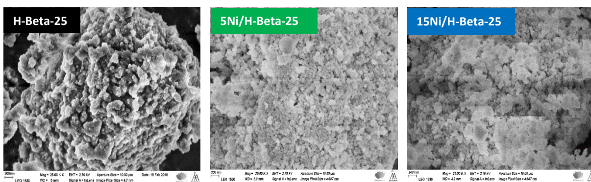
Figure 5.6. SEM images of H-Beta-25, 5Ni/H-Beta-25, and 15Ni/H-Beta-25. (The magnification of all images is 25.00 K X).
