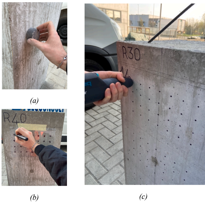
Fig. 5. Phases of the SH test: (a) smoothing of the surface; (b) drawing of the test points; (c) execution of the test.
