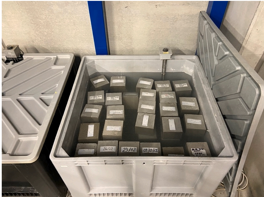
Fig. 2. Cube specimens inside the curing tank.
