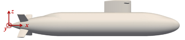
Fig. 1. Lateral view of the BB2 submarine and frame of reference.
