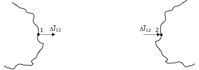
Fig. 6. Current injections -\Delta \bar{I}_{12} and \Delta \bar{I}_{12} into the two ends of the target line.
