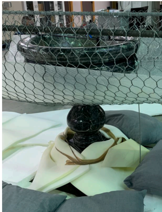
Fig. 6. Force application on the holy water stoup during the loading test.
