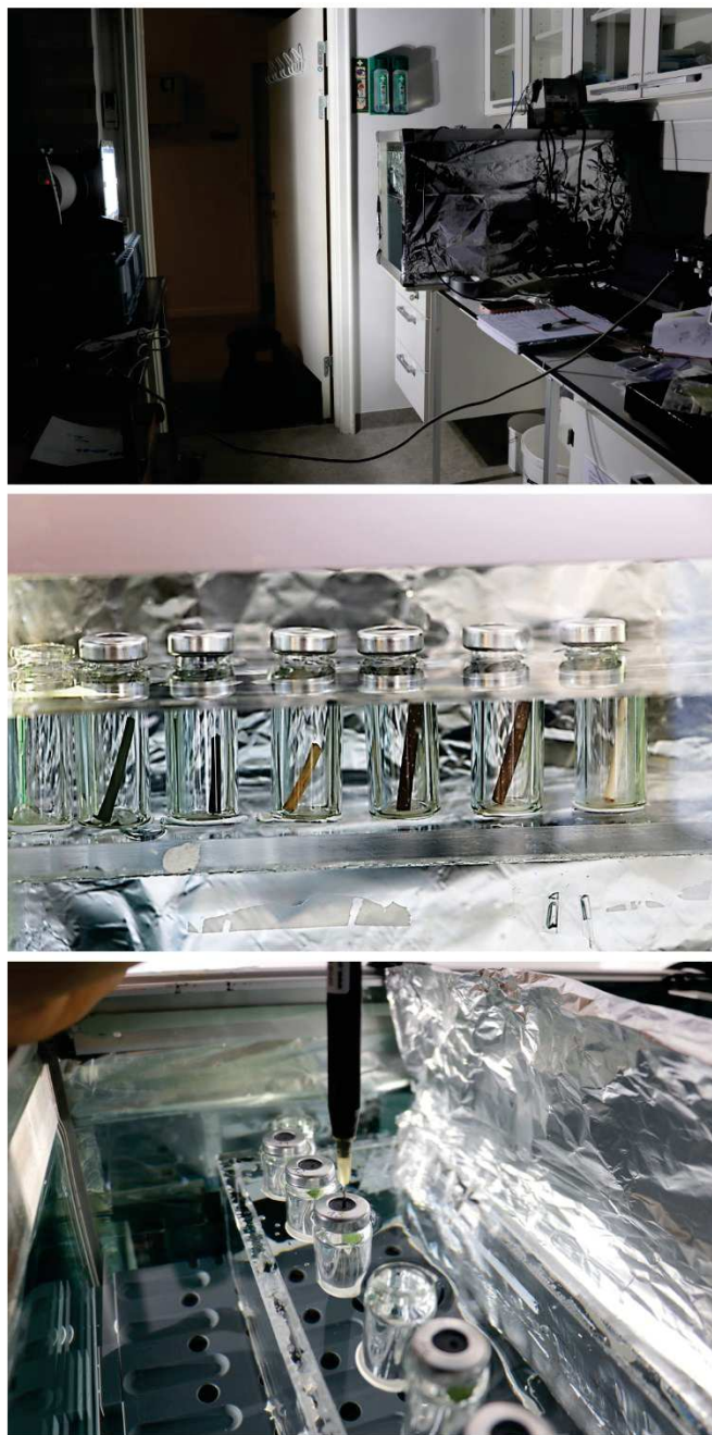
Fig. S1 Photograph of the experimental MicroRespiration setup.
