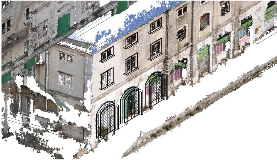
Figure 32: Modelling from point cloud reference
