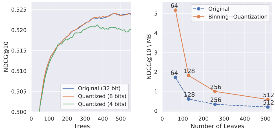
Figure 6.12: \lambda -MART efficiency/effectiveness trade-off. Right: NDCG@10 per MB of model size. Left: impact of quantization on NDCG@10. From [249].
