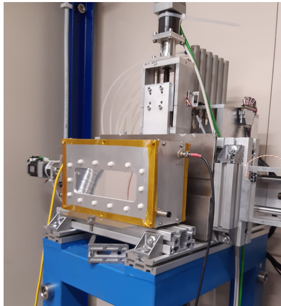
Figure 3.10: An image of one of the two custom-made ionization chambers to monitor the beam placed ahead from the breast sample. Original photo taken by the author.
