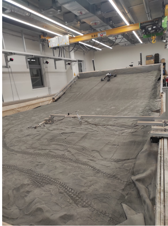
Figure 2.41: Experimental setup of the DLR PEL sandbox and the rover climbing a 20° slope.
