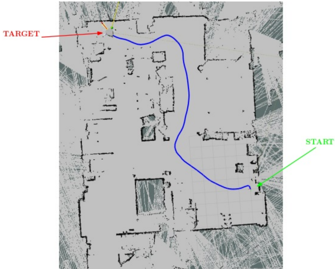
Figure 3.36: Trajectory of the mobile robot for the point-to-point motion in the absence of dynamic obstacles [366].
