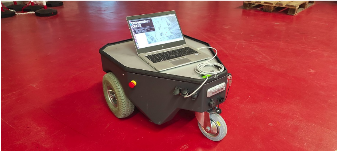
Figure 3.32: The elected differential drive mobile robot used in the experimental campaign: a Neobotix MP-500 [366].
