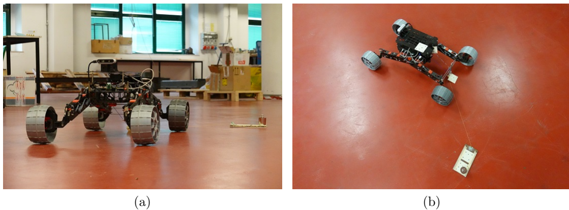
Figure 2.62: Experimental test of the rover Archimede towing an unbalanced object from a front three-quarter view (a) and a top view (b).
