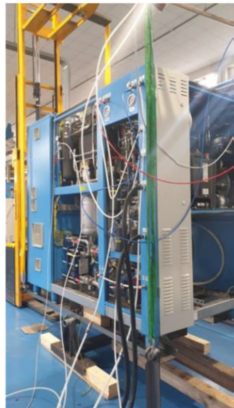
Figure 61. Alkaline Electrolyser on tilting plane during test. [98]
