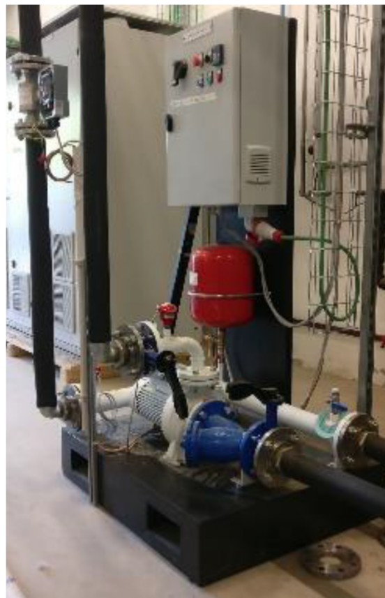
Figure 74. Fuel cell external cooling circuit pump skid installed in the test rig. Photo by the author.
