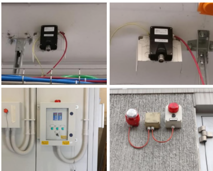
Figure 115. Test rig. Hydrogen detection system. [94]
