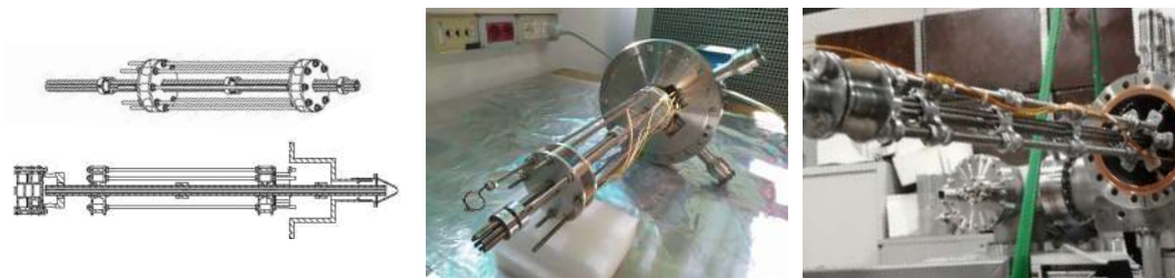
Figure 2.4: Technical drawing (left) and photographs of the first (center) and second (right) octupoles.
