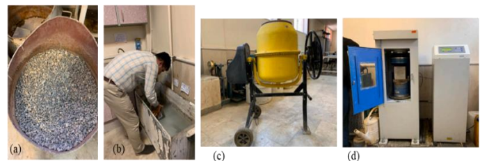
Fig. 3 Test setup (a) aggregate, (b) concrete mixture, (c) curing phase, (d) compressive strength test.
