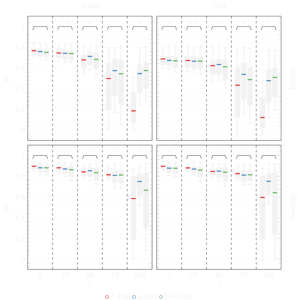
Fig. 6. Distribution of R^2 for different levels of \tau on training and test sets w.r.t. the different simulated user profiles. For each \tau statistical significance is reported.
