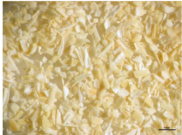
Figure 77: Stereoscopic microscopy images of raw (A) and delignified (B) milled rice husk, particle size 200-400 \mu\text{m} .
