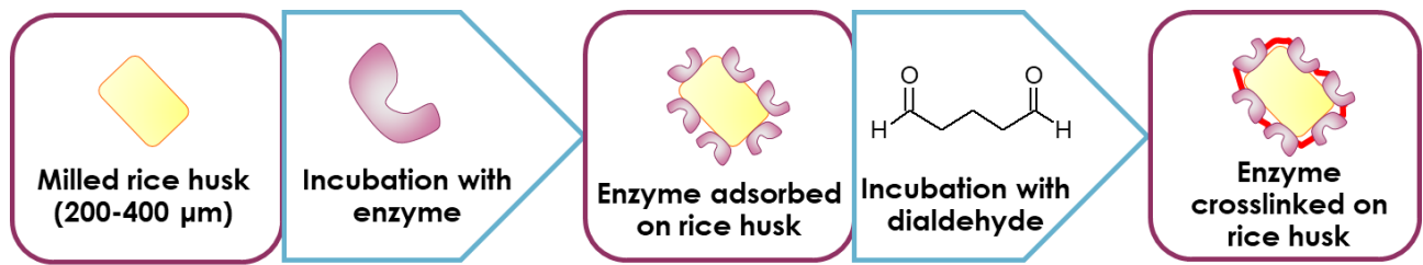
Figure 89: Schematic representation of the procedure for the adsorption and crosslinking of enzymes on rice husk
