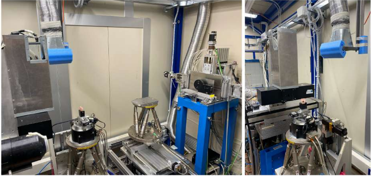
Figure 4.1: Experimental hutch of the SYnchrotron Radiation for Medical Physics (SYRMEP) beamline at the Italian synchrotron Elettra.
