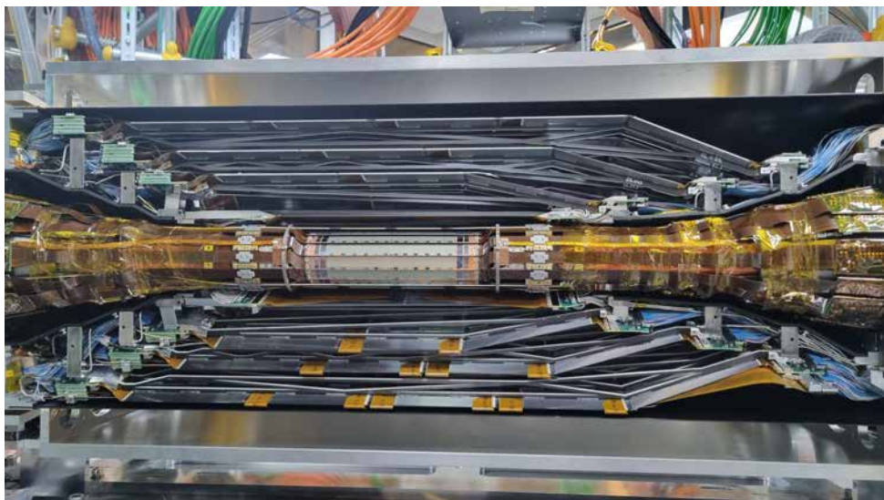
Figure 2.13: First half of SVD attached to PXD2.
