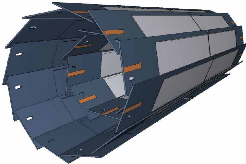
Figure 2.5: Schematic view of the geometrical arrangement of the PXD sensors. The light grey surfaces are sensitive DEPFET pixels [16] thinned to 75 \mu\text{m} .
