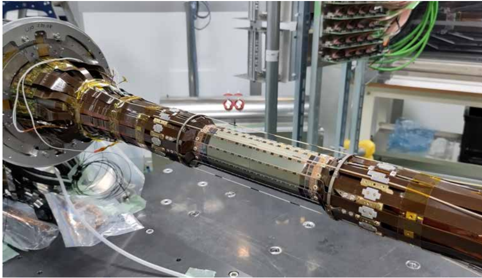
Figure 2.12: PXD2 after the installation on the beam pipe.
