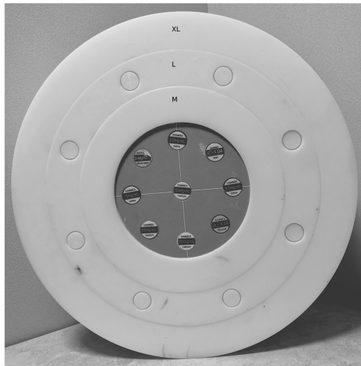
Figure 28: The phantom with inserts used for data collection. The core is a commercial Multi-Energy CT Phantom (Model 1472, Gammex Inc.) while fat-equivalent rings were produced in-house to simulate different patient sizes.
