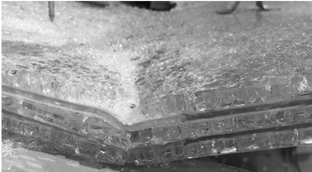
Figure 2. Post-breakage stage for a 3-ply LG element in laboratory test setup.
