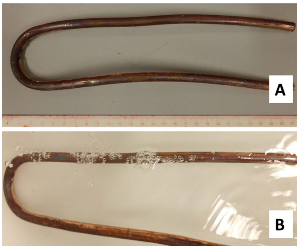
FIGURE 1 | Failed pipe section as cut (A) and the same failed pipe section during the pressure test (B). The exact location of leakage due to microscopic holes (not visible in A) is pinpointed by the air bubbles in B. [Color figure can be viewed at wileyonlinelibrary.com ]
